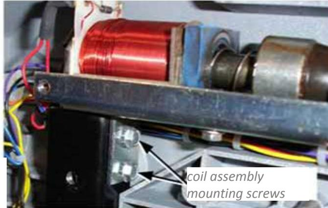
*coil assembly mounting screws*
