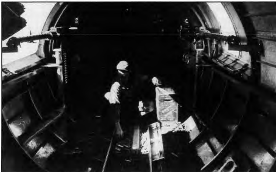
At the end of a mission a member of the ground crew picks up spent cartridge cases scattered around the waist guns of a Fortress. The two Browning 0.50 calibre machine guns are in their post mission positions.
