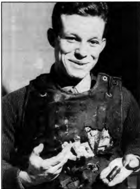
The flak vest stopped a 20mm incendiary shell worn the waist gunner. He was knocked breathless but recovered and later shot down two enemy fighters.
