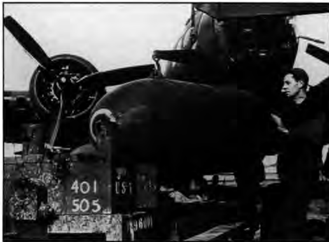
Loading a big bomb from the trailer to a cradle prior to being fitted into the bomb bay of the B-17F.
