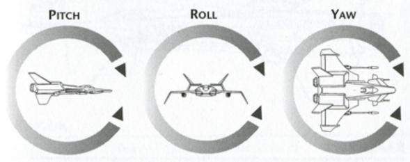
Pitch. Ability of a ship to change direction up or down.
