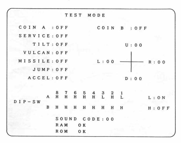
To test the game sounds, move the control grip to the right or left until the desired sound address appears next to the SOUND CODE display. Then press the MISSILE button to activate that sound.
