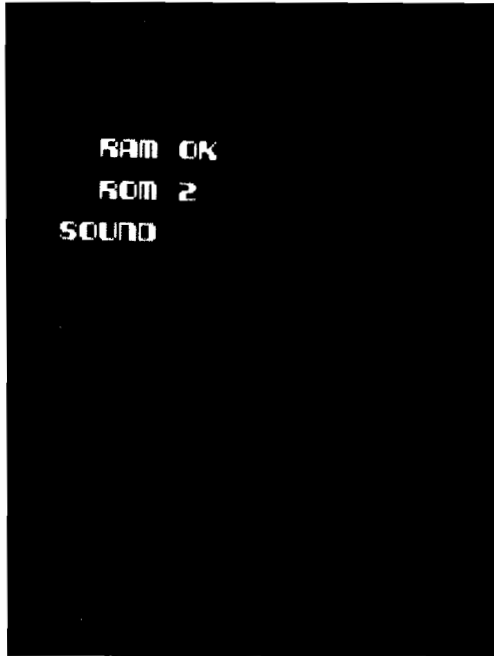
Figure 2-3 Self-Test Display (ROM Failure)
